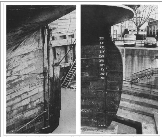
The photograph on the left shows the jury rudder that was installed on the *Cutty Sark* while at sea in 1872. The recent photograph (right) provides some perspective on the size of the rudder.
